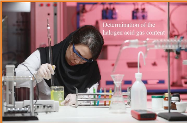
Determination of the halogen acid gas content
